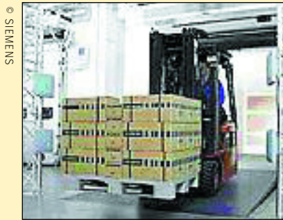
The Simatic RF 600 utilizes UHF technology to allow longer distances between readers and RFID tags attached to products or items, at low costs.
